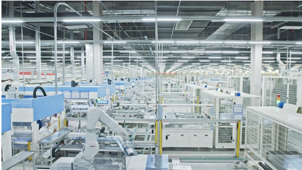
Figure 3-17: Highly automated solar module assembly facility. 103
